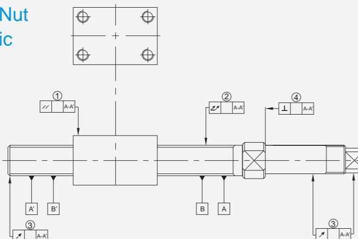
GMT makes the necessary inspection of geometric tolerance as the following items:
