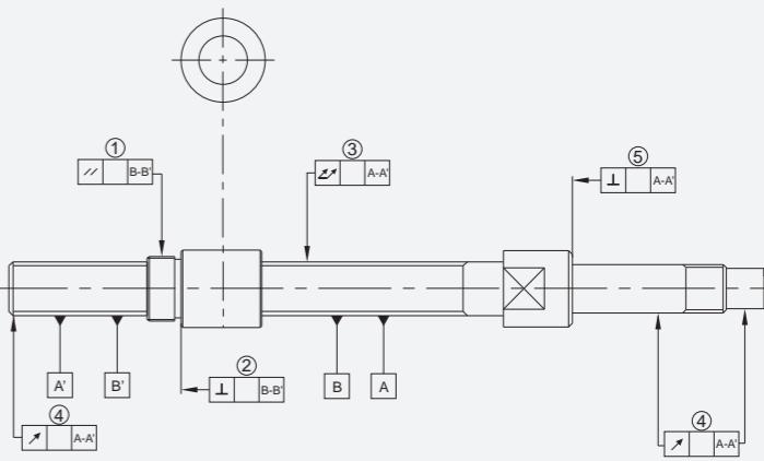
GMT makes the necessary inspection of geometric tolerance as the following items:
