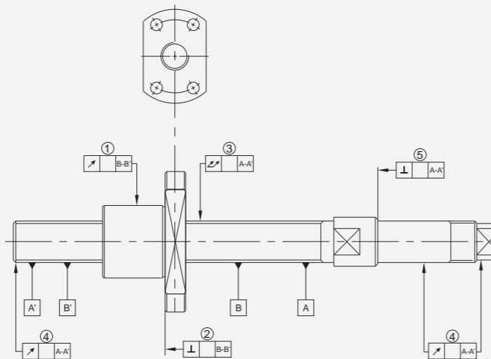
GMT makes the necessary inspection of geometric tolerance as the following items:
