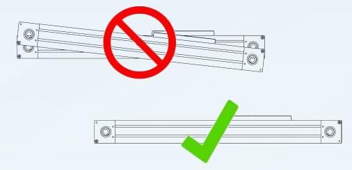
Actual tolerances related to alignment recommendations and mounting vary from actuator series. Profile ball rail systems tend to be quite rigid and alignment is more critical. Guide wheel units often have clearance, which offer some forgiveness in alignment.
