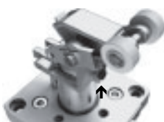
Sensing of the toggle lever position
