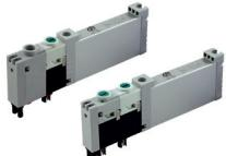
Solenoid valves size 10 mm with sub-base connections for valve terminals series A5, available in functions 5/2 solenoid/spring and 5/2 solenoid/solenoid. Easy and practical mounting, low consumption coils (1,2W), 360° view LED and equipped with "push" and bistable manual override. Compatible with sub-bases size 10 mm and with all the communication interfaces.
