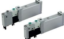
Solenoid valves size 14 mm with sub-base connections for valve terminals series A5, available in functions 5/2 solenoid/spring and 5/2 solenoid/solenoid. Easy and practical mounting, low consumption coils (1,2W), 360° view LED and equipped with "push" and bistable manual override. Compatible with sub-bases size 14 mm and with all the communication interfaces.
